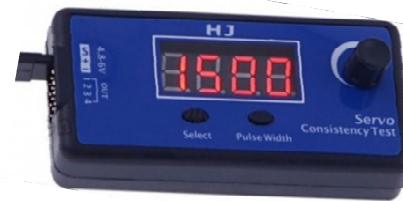
HJ servo tester displays pulse widths directly in \mu\text{s} .
