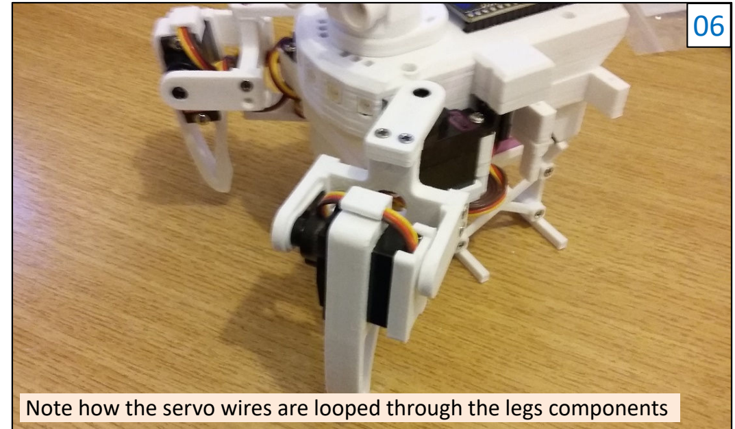
Ensure the legs and wires can move freely.
